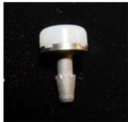
**Figure 1. UHMWPE-HA Microcomposite on Titanium Stem.**
