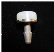
**Figure 1. UHMWPE-HA Microcomposite on Titanium Stem.**
