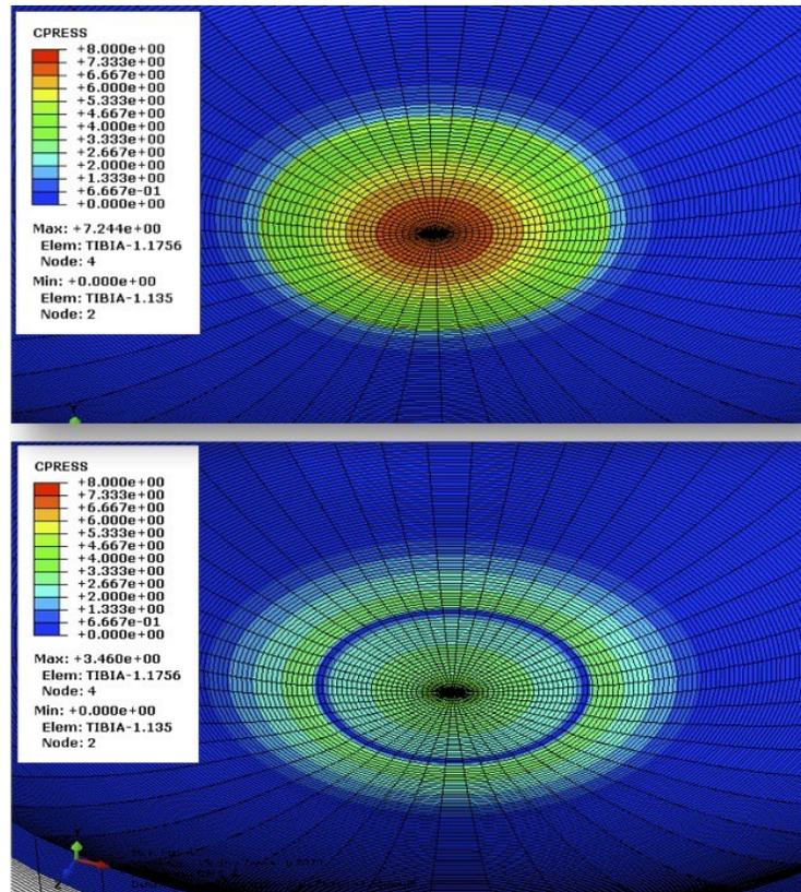
**Pressure mapping looking at metal implant on tibial cartilage contact pressures, peak 7.24MPa, active contact zone loaded area - 314mm<sup>2</sup> and BioPoly implant on tibial cartilage contact pressures, peak 3.46MPa, active contact zone loaded area - 471mm<sup>2</sup>.**
